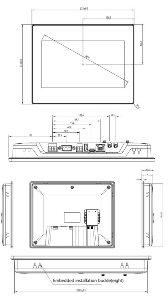
Flush-mounted installation cutout dimensions:260mm\*202mm(+1.5mm/-0.0mm)
